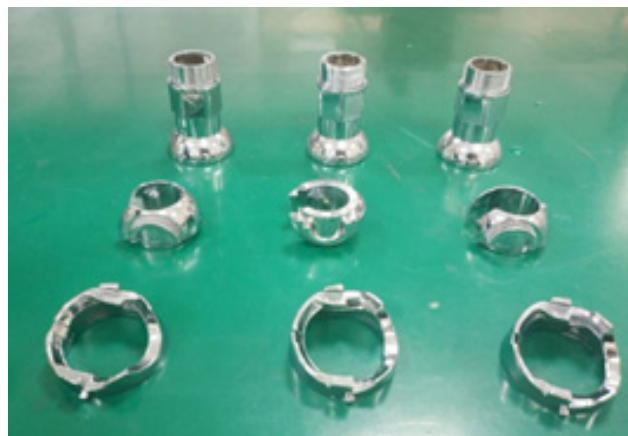
Figure 3.6 Samples after NEMA-4X salt spray test
