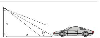
In both the vertical and the horizontal placement, the angle between the camera lens and the farther lane border must be less than 30°. Ensure the snapshot distance (x) of the camera is greater than 1.7 times the height (h) of the camera ( $x \ge 1.7 \times h$ ) for optimal license plate images.
