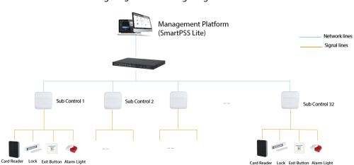
Figure 3-1 Networking Diagram
